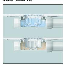
Fig. 1: Mode of operation of the odour trap
