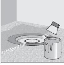
Lay the sealing collar into the bonded sealing.
