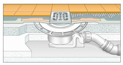
Fig. 4: Diagram of a bonded seal
