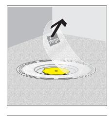
Apply the bonded sealing on the dry screed and spread to the inner edge of the flange fleece.
