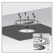
Screw the sealing flange together tightly with the drain.
