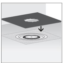
INFO! The Viega sealing collar has two differently coated sides. One side is coated with bitumen and the other side with EPDM. If the additional sealing takes place with bitumen sealing lanes, the sealing collar must be used with the bitumen side facing upwards. If EPDM sealing lanes are used, the EPDM side must face upwards.
