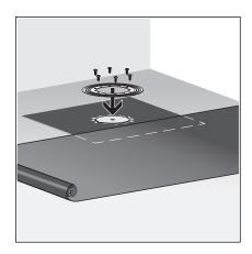
Position the sealing flange on the sealing collar in such a way that the screw holes are visible.
