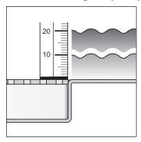
Drainage capacity at an accumulation height of 20 mm above the grate: 0.4 l/s
