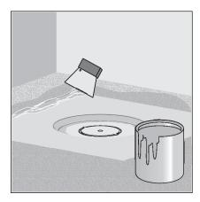
Apply a second layer of bonded sealing onto the sealing collar and, if necessary, onto the floor.
