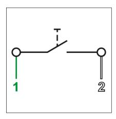
Fig. 4: WC flush plate, terminal assignment for external sensors
